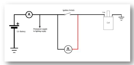
This simplified diagram is not intended to be used as an instruction for connecting the alternator. Rather it is to demonstrate the function of the two wires from the alternator.
