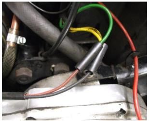
The black outut wire connects to the yellow dynamo wire in the loom. The red alternator battery sense and field coil wire connects to the green dynamo field coil wire in the loom.
