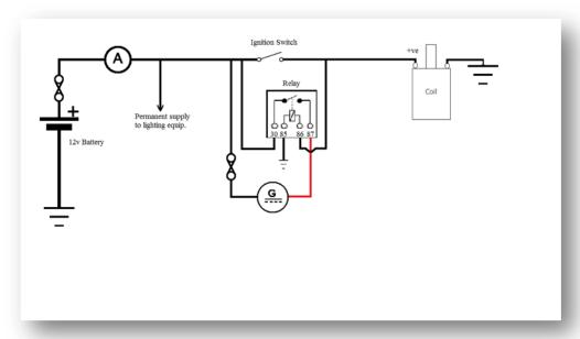
In this circuit a relay is used to connect the red field coil/battery sense wire to the system +ve. When the ignition switch is closed the relay coil is energised and the contacts in the relay close. The connection from pin 30 on the relay will probably be best joined into the loom at the same point as the generator output wire.
