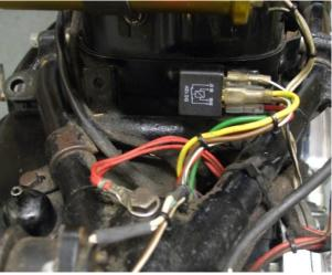
The regulator is removed and the all the wires are connected to the relay as per the diagram below. An additional feed is taken from the ignition switch to energise the relay.
