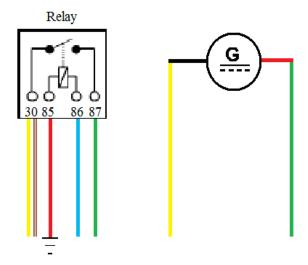
In the diagram above the wires to relay are the ones removed from the regulator except for the blue wire which is a feed from the switched side of the ignition switch to energise the relay. The yellow and brown/wire are connected together at terminal 30 (put them both into a single female spade terminal) this takes the output from the alternator to the battery.
