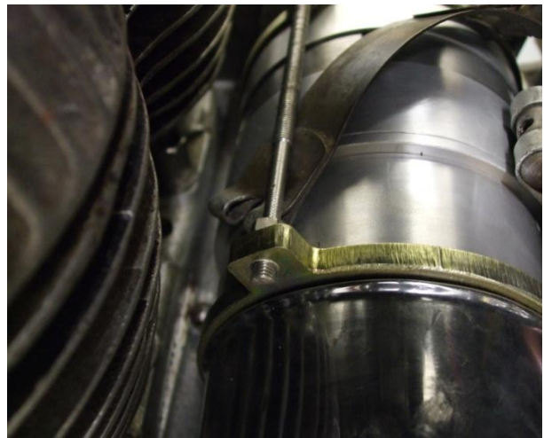
The domed nut removed to allow top strap to pass between threaded rod and case.
