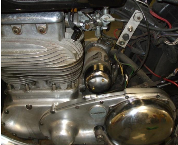
Drive side prepared for dynamo removal
