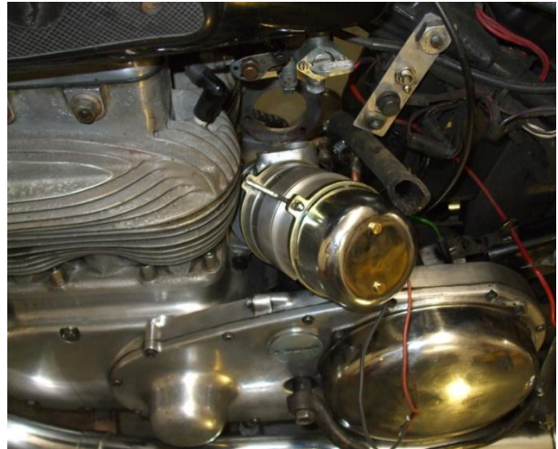
Inserting the alternator. Start from this position and gradually straighten.
